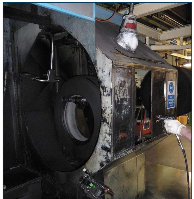
Figure 8 Enclosed and exhausted spray booth for controlling solvent mist and vapours
