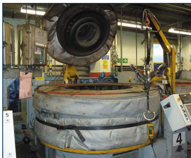
Figure 4 Tyre press fitted with safety trip device
