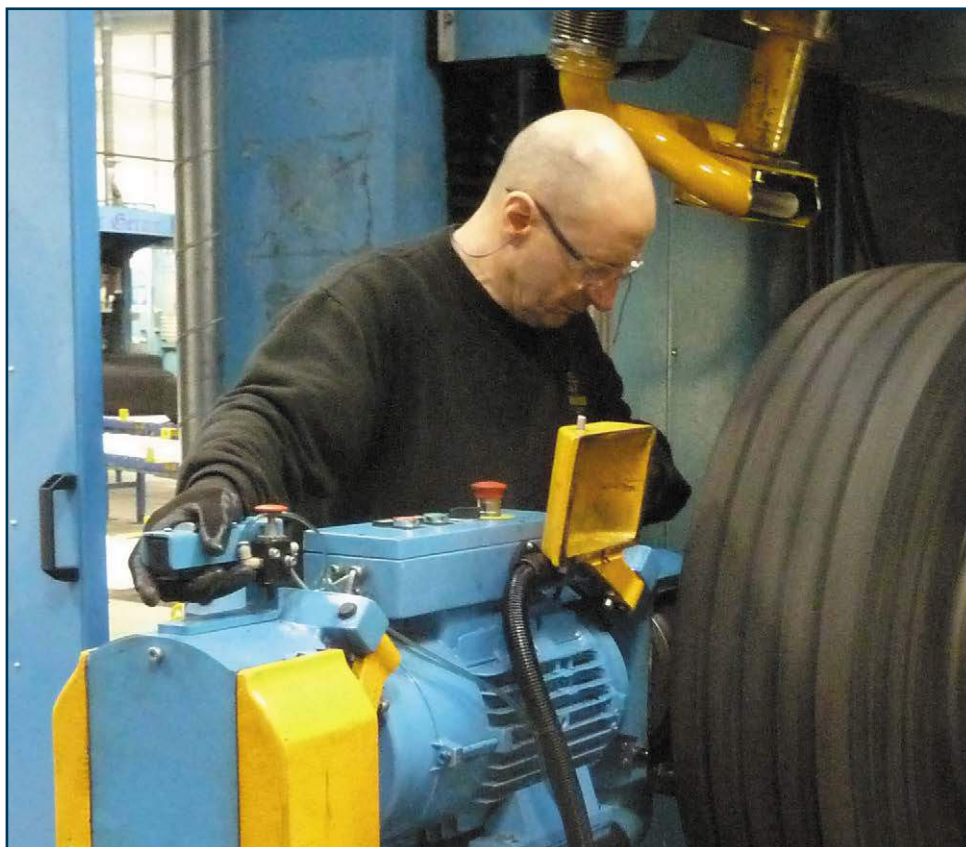
Figure 2 Articulated-head buffing machine with two-hand control
