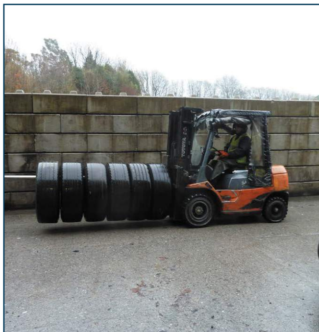
Figure 12 Fork Truck fitted with carpet Pole
