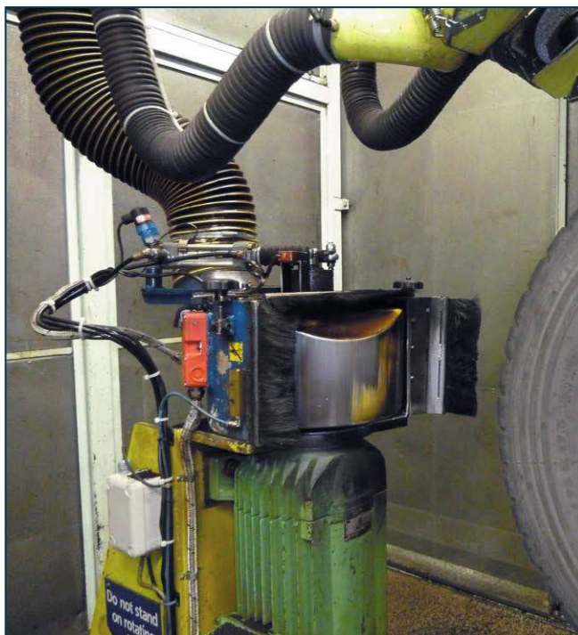
Figure 6 Buffing machine rasp housing fitted with LEV
