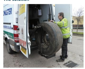
Fit a ramp to the recovery vehicle to help with loading and unloading of tyres. Provide a tail or side lift to load and unload tyres. This is especially important if handling tyres from commercial, agricultural or earth-moving equipment. Avoid raising the heaviest tyres from the floor to the vertical whenever possible. Fit the tyre without removing the wheel from the vehicle.
